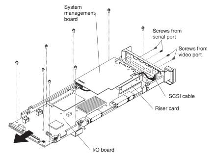
13. Remove the riser card from the I/O board, disconnecting any cables.
